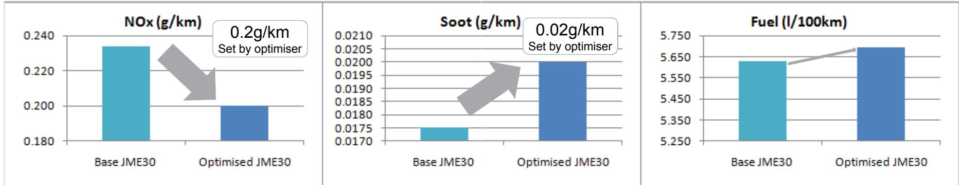
Baseline calibration emissions on JME30 were characterised by relatively high NOx and low soot
