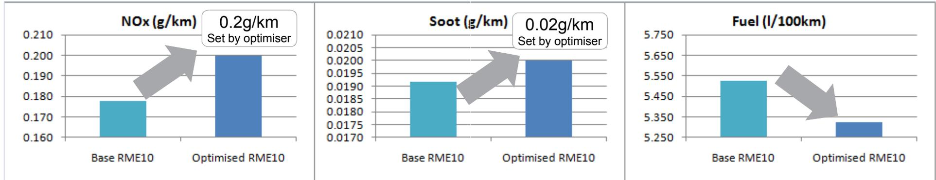
Low NOx and soot levels on the baseline calibration for RME10 enabled a low FC solution to be found by the optimiser
