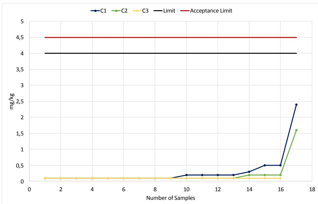
Diagram 15: Phosphorus Content according to DIN EN 14107 / Campaigns 1 to 4
