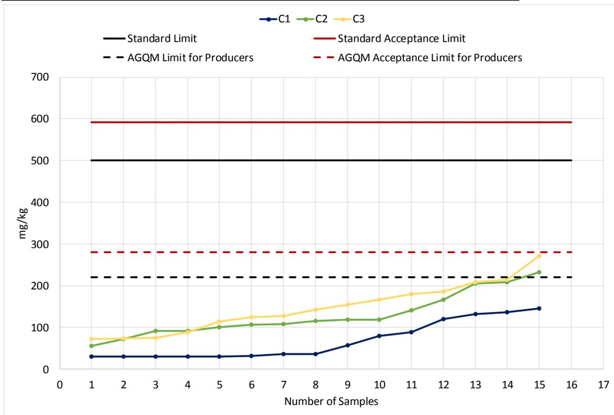
**Diagram 4: Water Content according to DIN EN ISO 12937**
