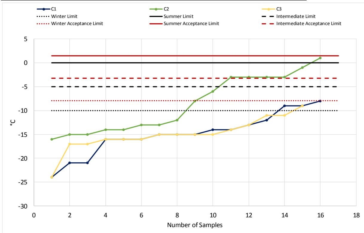
**Diagram 17: CFPP according to DIN EN 116**
