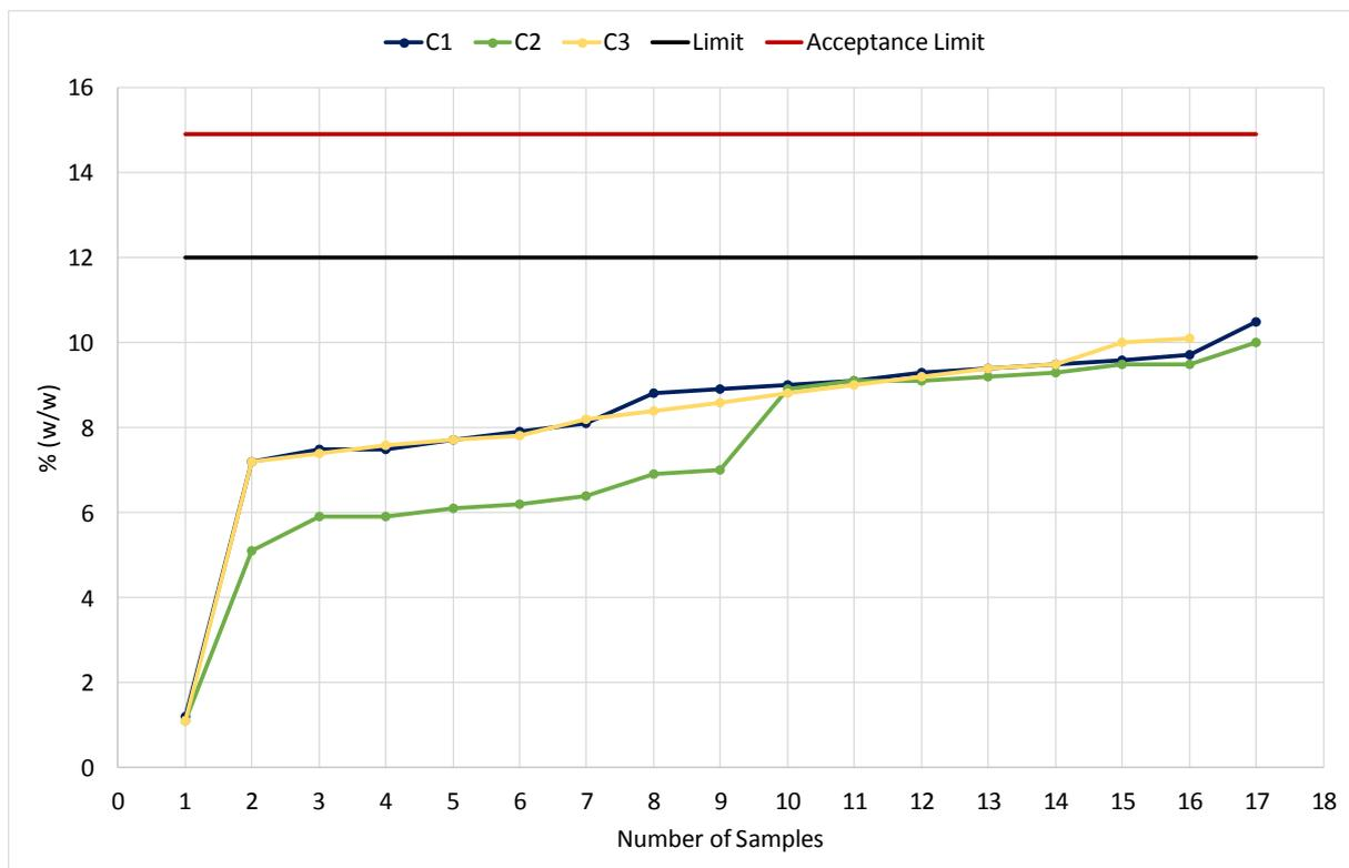
**Diagram 16: Content of Linolenic Acid Methyl Ester according to DIN EN 14103**
