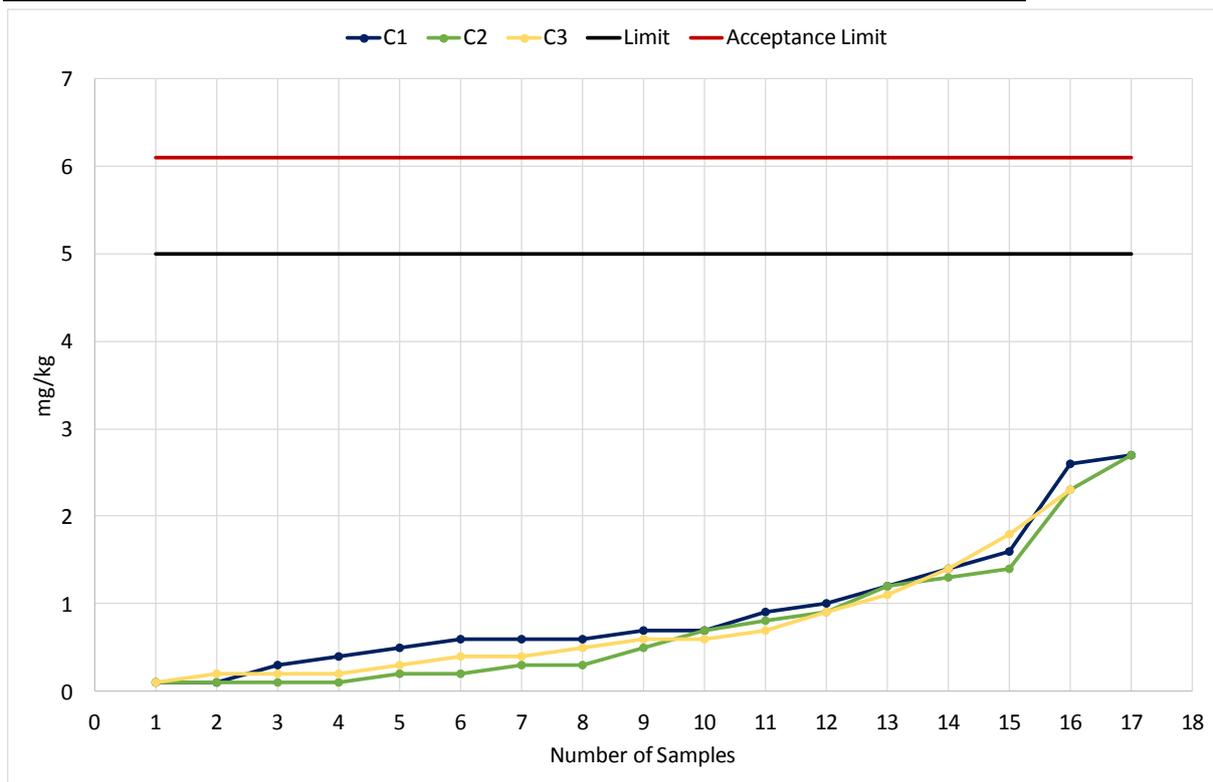
Diagram 13: Sum of Alkali Metals Sodium and Potassium according to DIN EN 14538
