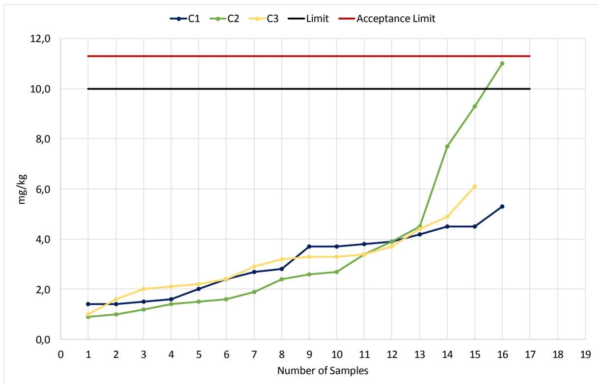
Diagram 3: Sulphur Content according to DIN EN ISO 20846
