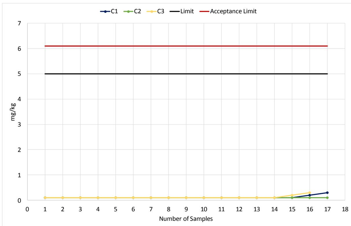
Diagram 14: Sum of Earth Alkali Metals Calcium and Magnesium according to DIN EN 14538
