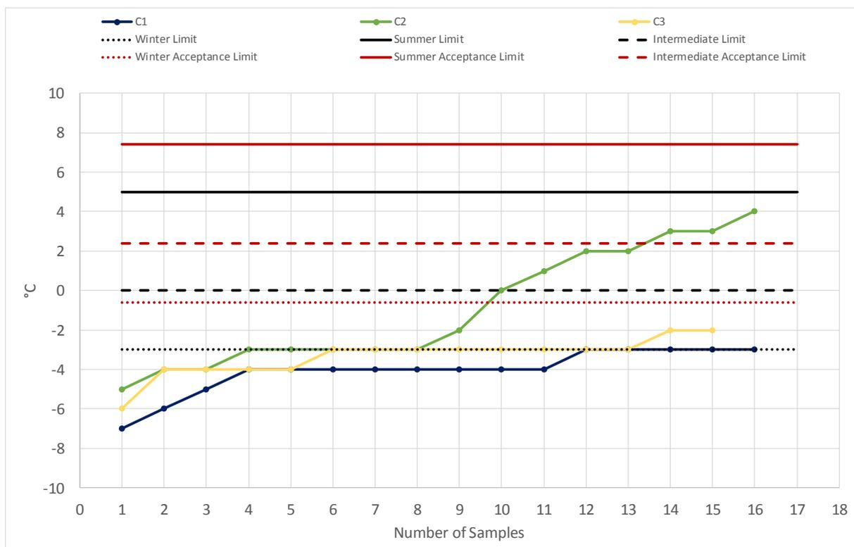
Diagram 18: Cloud Point according to DIN EN 23015
