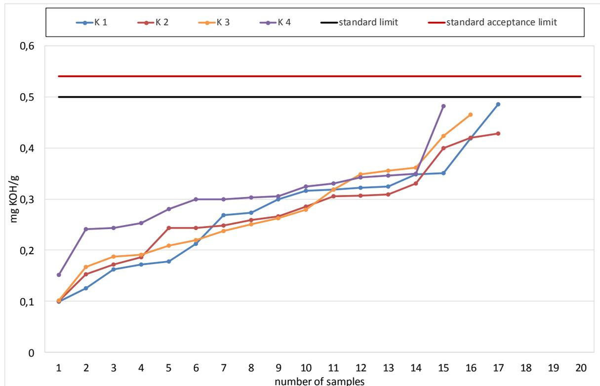
**Diagram 7: Acid Number according to DIN EN 14104.**
