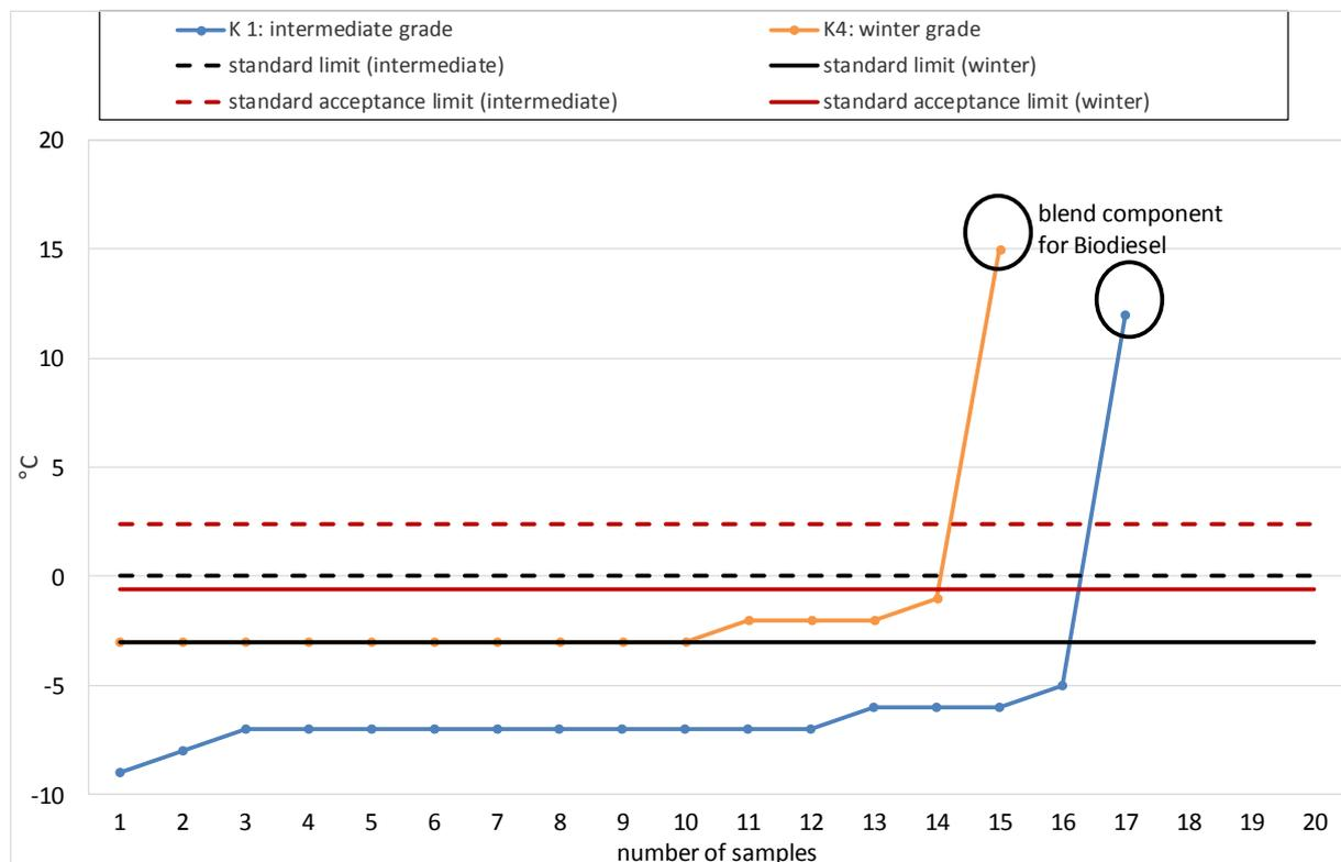
**Diagram 20: Cloud Point (intermediate and winter grades) according to DIN EN 23015.**
