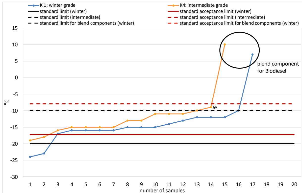
**Diagram 18: CFPP (intermediate and winter grades) according to DIN EN 116**
