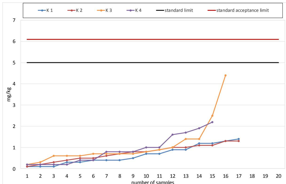
**Diagram 14: Sum of Alkali Metals Sodium and Potassium according to DIN EN 14538.**
