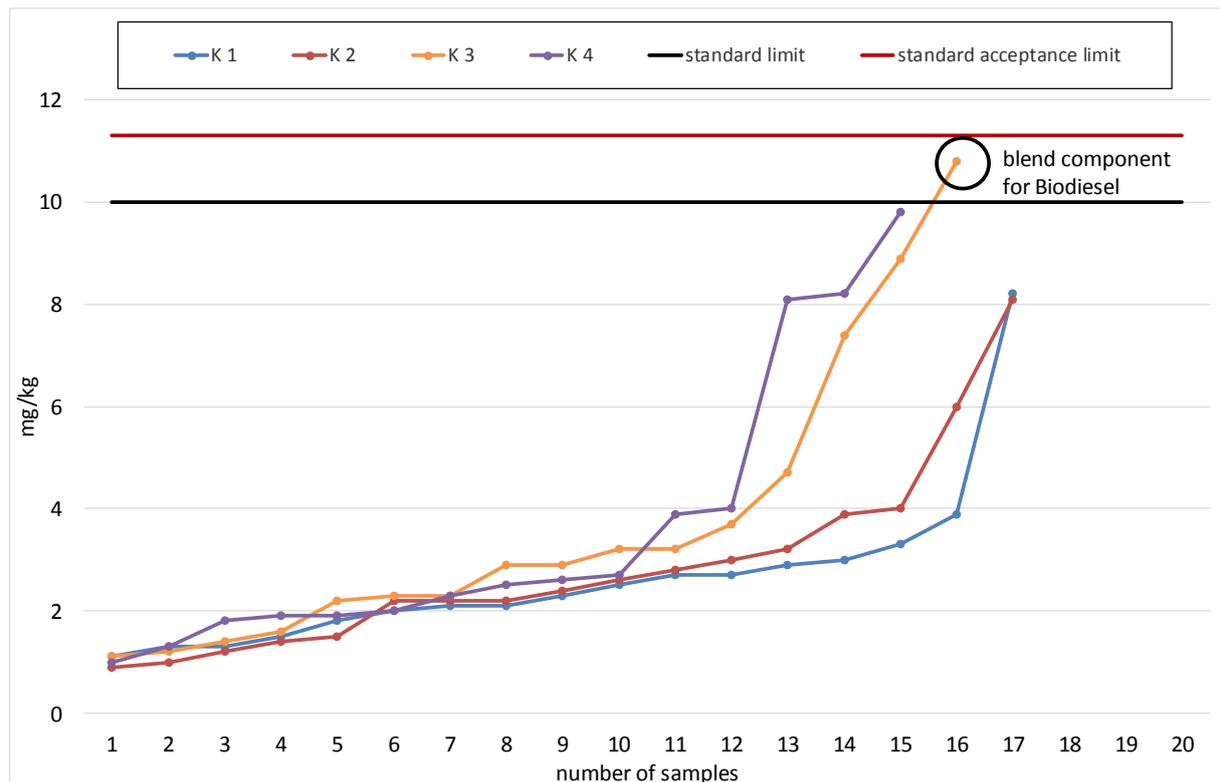
**Diagram 3: Sulfur Content according to DIN EN ISO 20846.**
