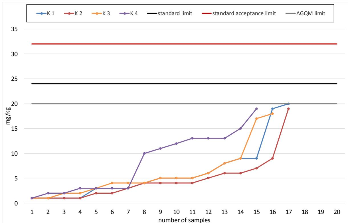
**Diagram 1: Total contamination according to DIN EN 12662.**
