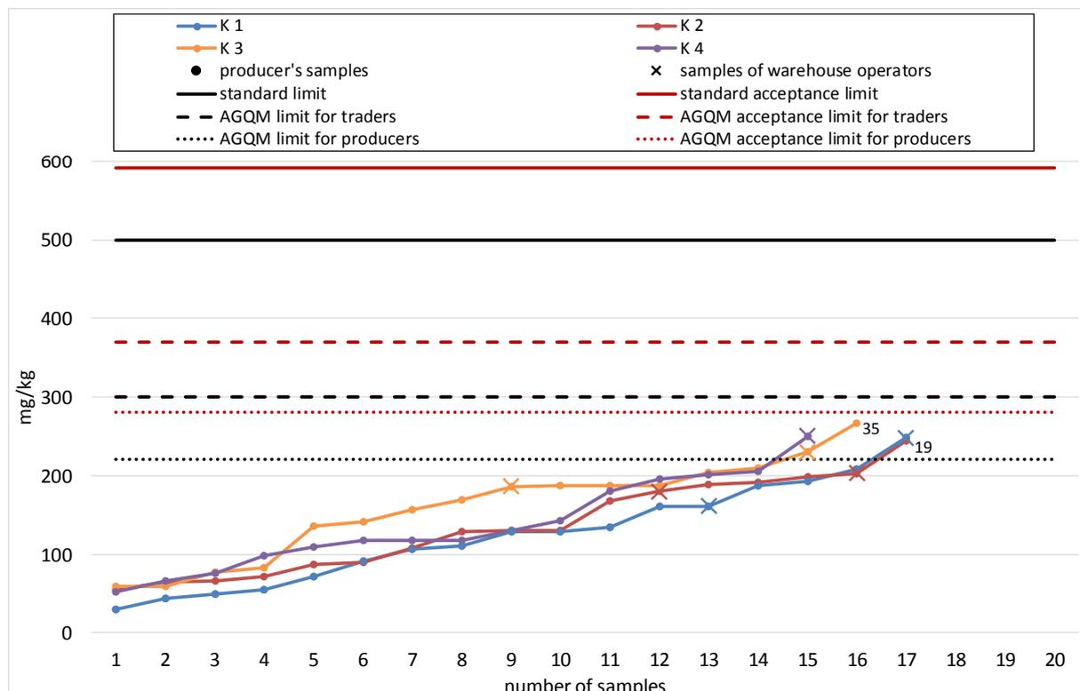
**Diagram 4: Water Content according to DIN EN ISO 12937.**
