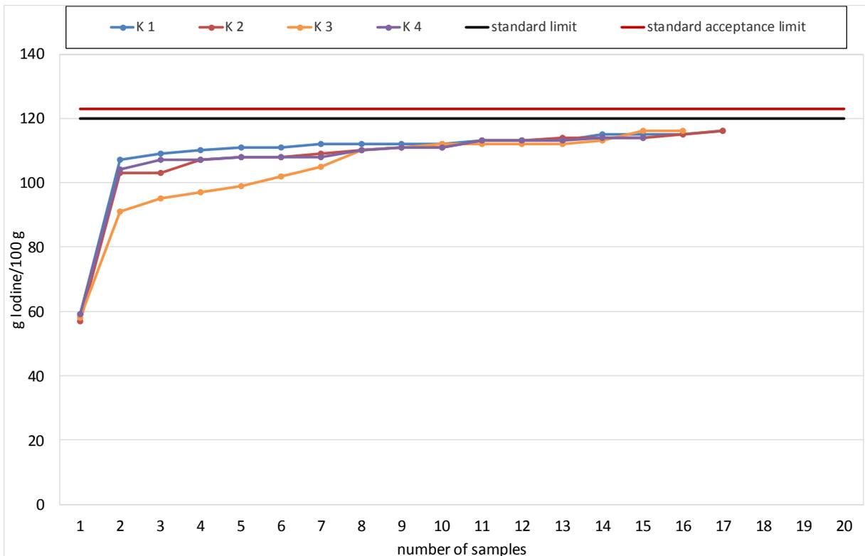
**Diagram 9: Iodine Number according to DIN EN 14111 (titrated).**
