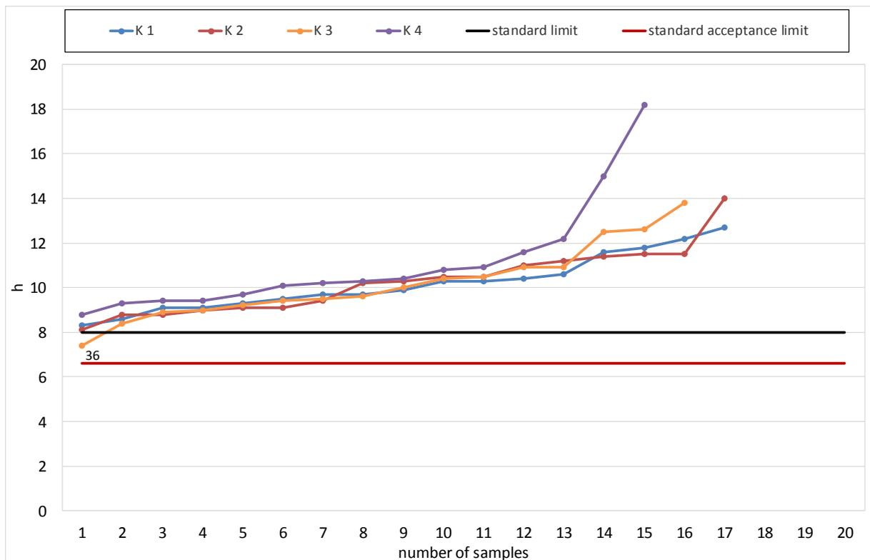
**Diagram 6: Oxidation Stability according to DN EN 14112.**
