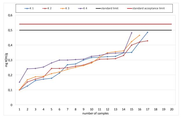
Diagram 7: Acid Number according to DIN EN 14104.
