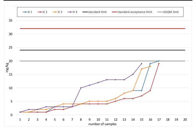
Diagram 1: Total contamination according to DIN EN 12662.
