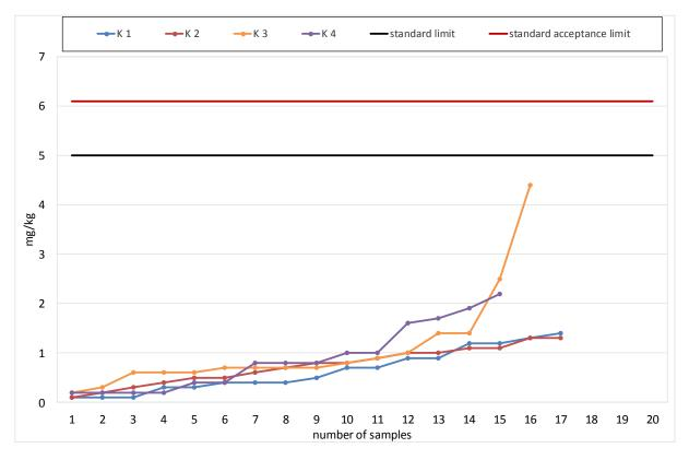
Diagram 14: Sum of Alkali Metals Sodium and Potassium according to DIN EN 14538.
