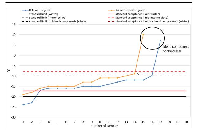
Diagram 18: CFPP (intermediate and winter grades) according to DIN EN 116
