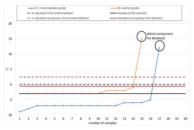
Diagram 20: Cloud Point (intermediate and winter grades) according to DIN EN 23015.
