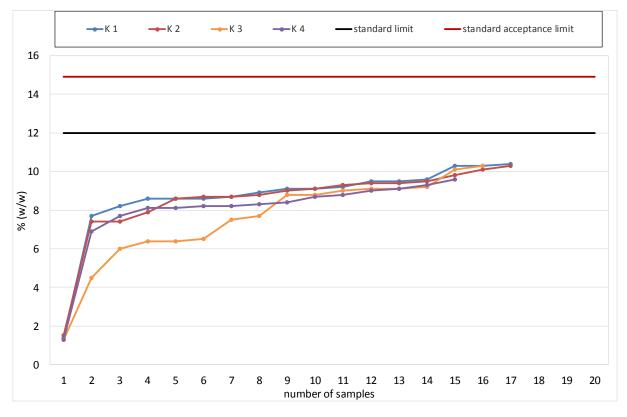
Diagram 17: Content of Linolenic Acid Methyl Ester according to DIN EN 14103.
