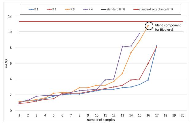
Diagram 3: Sulfur Content according to DIN EN ISO 20846.
