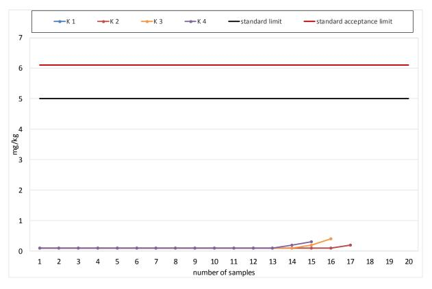
Diagram 15: Sum of Earth Alkali Metals Calcium and Magnesium according to DIN EN 14538.
