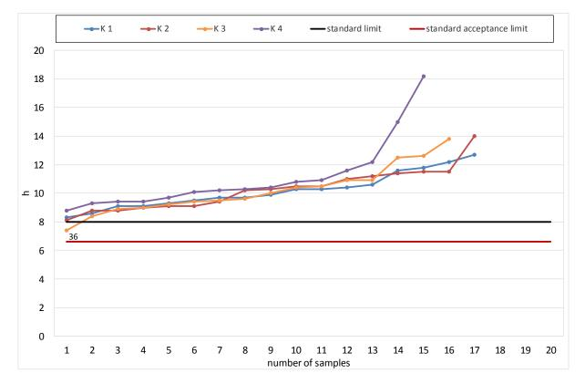
Diagram 6: Oxidation Stability according to DN EN 14112.
