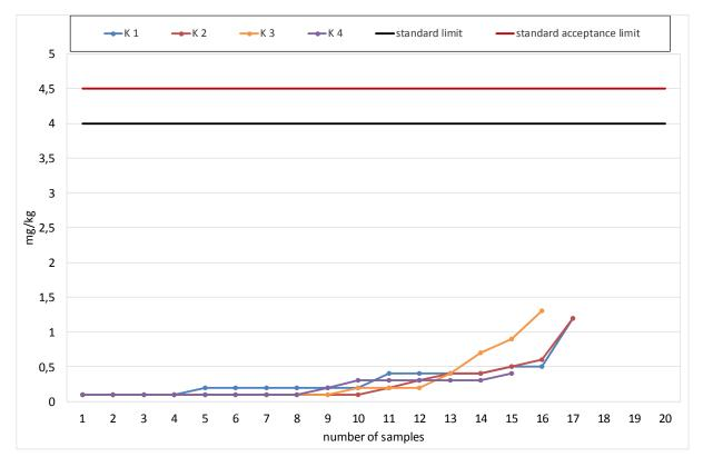
Diagram 16: Phosphorus Content according to DIN EN 14107, K2 to K4.
