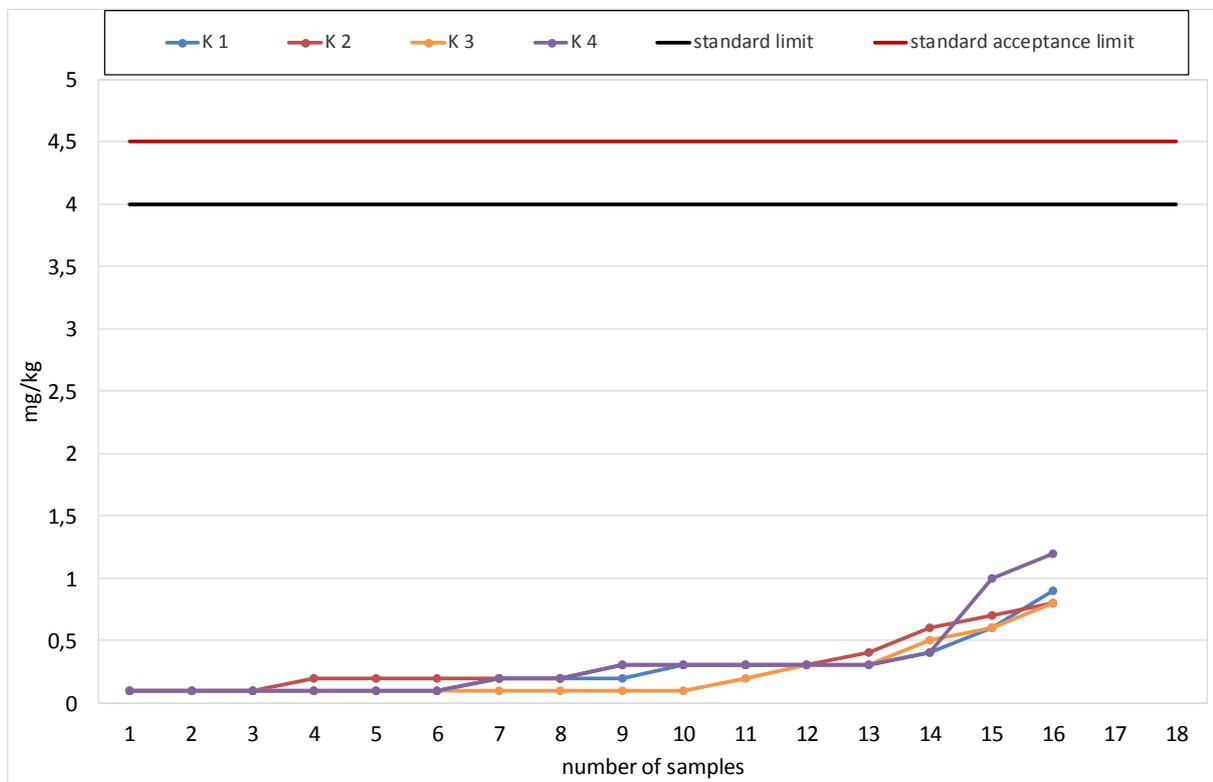
Diagram 16: Phosphorus Content according to DIN EN 14107.
