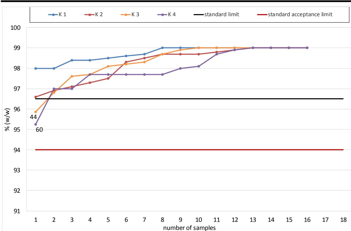
**Diagram 1: Content of fatty acid methyl ester according to DIN EN 14103.**
