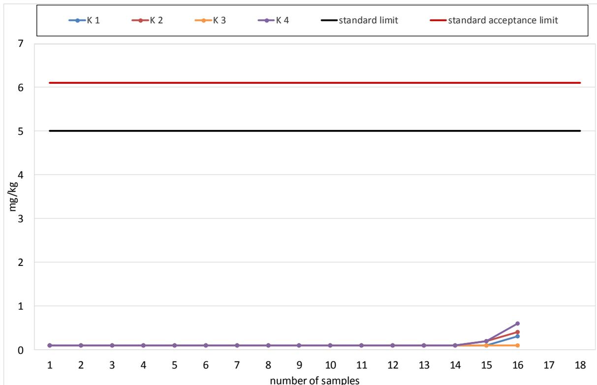
**Diagram 15: Sum of Earth Alkali Metals Calcium and Magnesium according to DIN EN 14538.**
