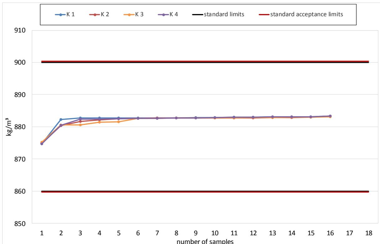
Diagram 2: Density at 15 °C according to DIN EN ISO 12185.
