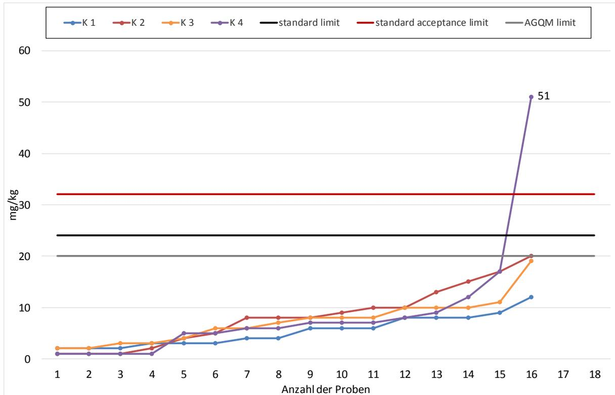
**Diagram 5: Total Contamination according to DIN EN 12662.**
