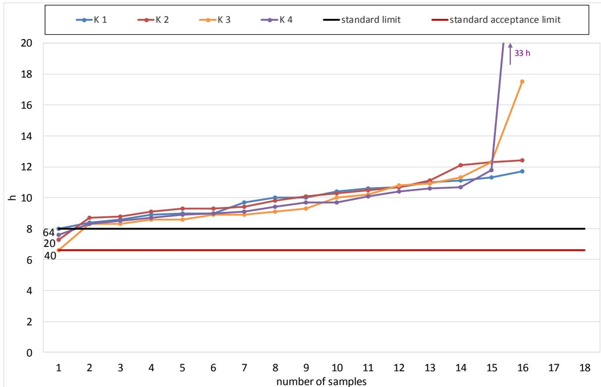
**Diagram 6: Oxidation Stability according to DIN EN 14112.**
