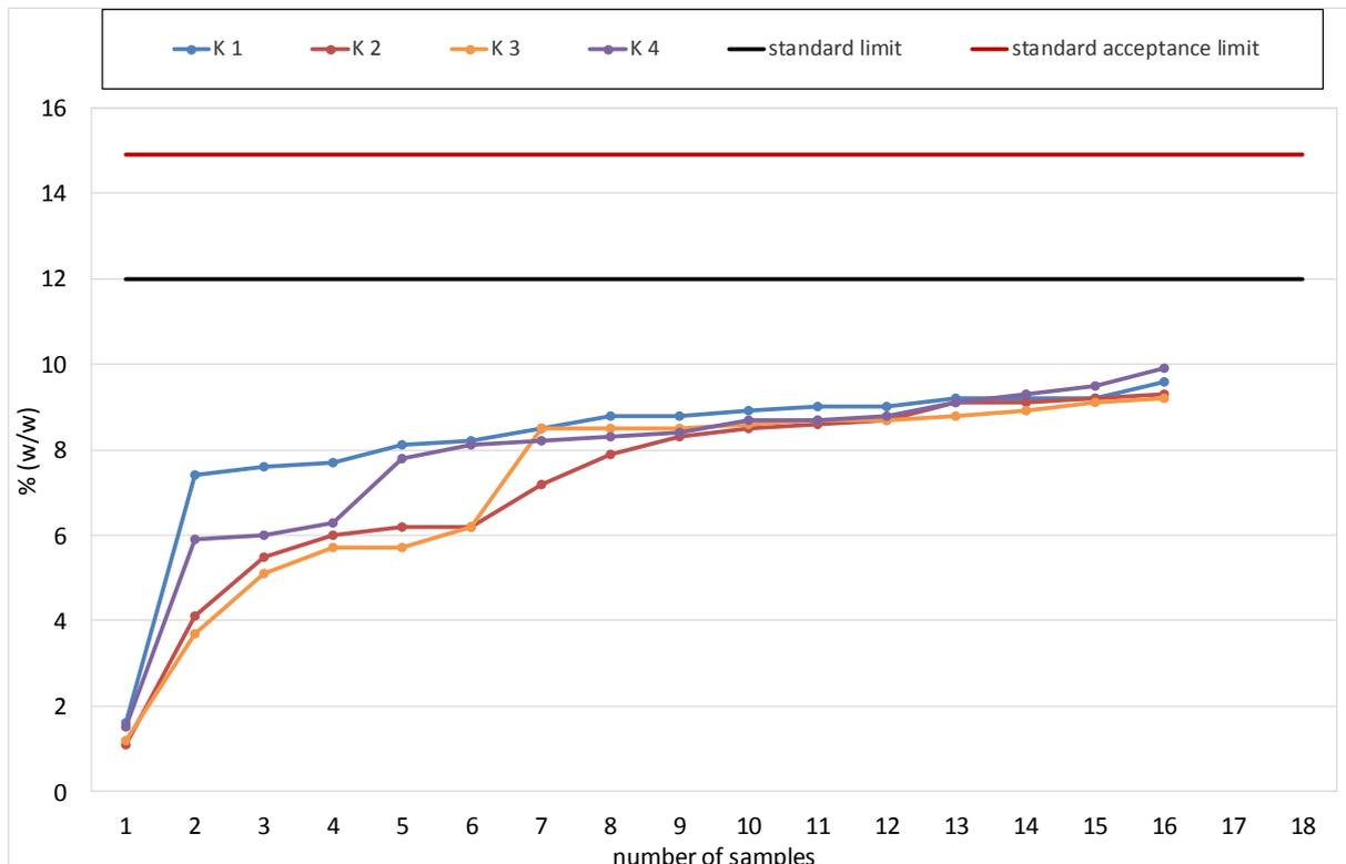
**Diagram 17: Content of Linolenic Acid Methyl Ester according to DIN EN 14103.**
