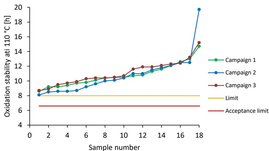
Figure 7: Oxidation Stability acc. to DIN EN 14112.
