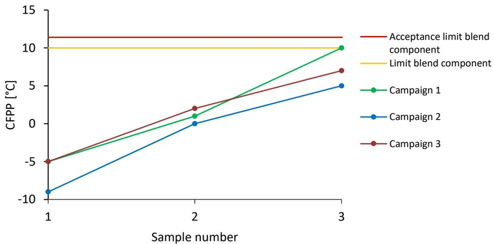
Figure 20: CFPP of blend components for biodiesel acc. to DIN EN 116.
