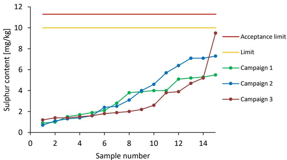
Figure 3: Sulphur content acc. to DIN EN ISO 20846.
