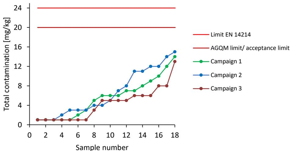
Figure 6: Total contamination acc. to DIN EN 12662.
