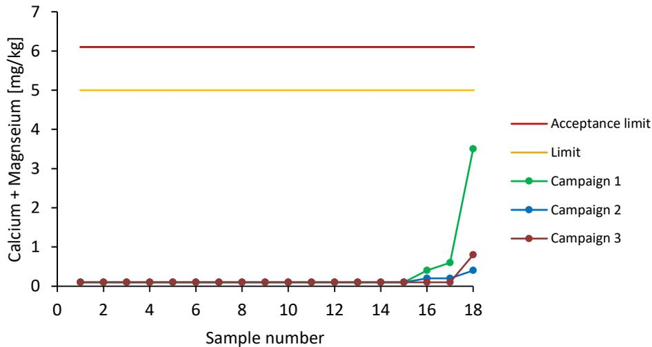
Figure 16: Sum of alkaline earth metals Calcium and Magnesium acc. to DIN EN 14538.
