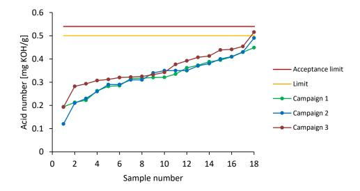
Figure 8: Acid Number acc. to DIN EN 14104.
