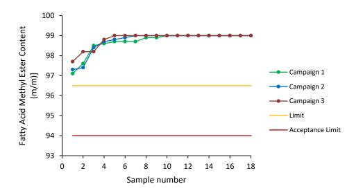
Figure 1: Fatty Acid Methyl Ester Content acc. to DIN EN 14103.
