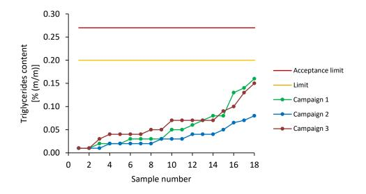
Figure 12: Triglycerides acc. to DIN EN 14105.
