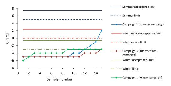
Figure 21: Cloud point acc. to DIN EN 23015.
