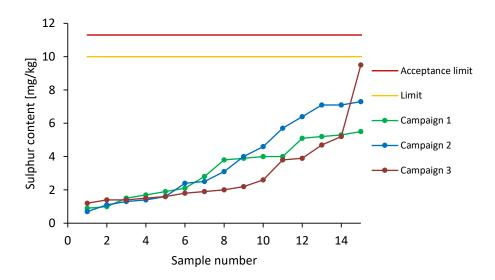
Figure 3: Sulphur content acc. to DIN EN ISO 20846.
