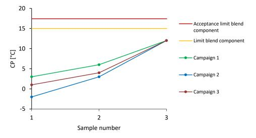
Figure 22: Cloud point of blend components for biodiesel acc. to DIN EN 23015.
