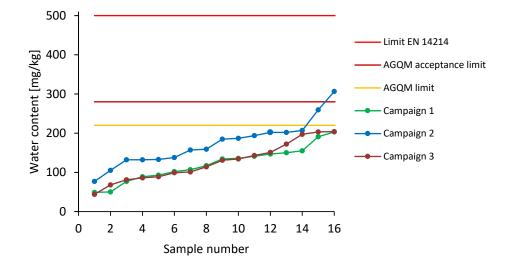
Figure 5: Water content acc. DIN EN ISO 12937.
