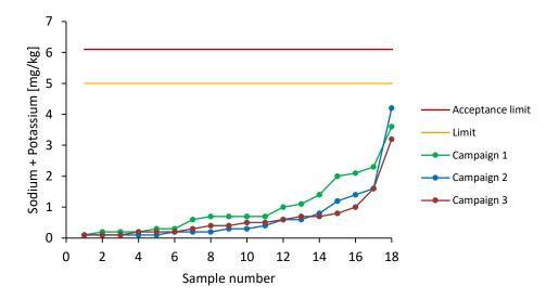
Figure 15: Sum of alkali metals Sodium and Potassium acc. to DIN EN 14538.
