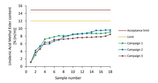
Figure 18: Content of Linolenic Acid Methyl Ester acc. to DIN EN 14103.
