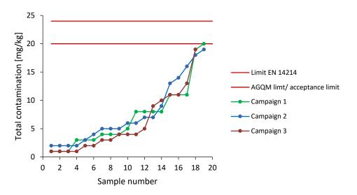
Figure 6: Total contamination acc. to DIN EN 12662.
