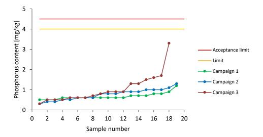
Figure 17: Phosphorus content acc. to DIN EN 14107.
