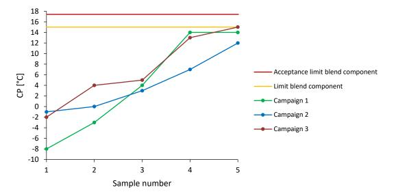
Figure 22: Cloud point of blend components for biodiesel acc. to DIN EN 23015.
