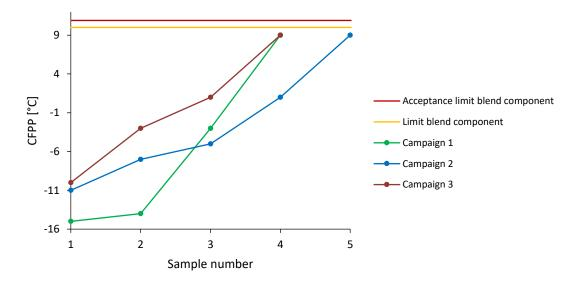
Figure 20: CFPP of blend components for biodiesel acc. to DIN EN 116.
