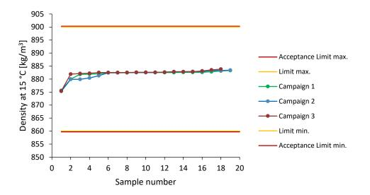
Figure 2: Density at 15 °C acc. to DIN EN ISO 12185.
