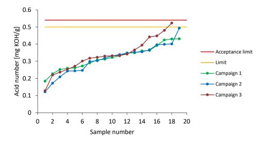
Figure 8: Acid Number acc. to DIN EN 14104.
