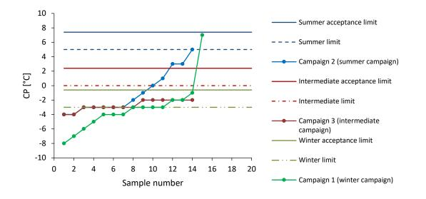
Figure 21: Cloud point acc. to DIN EN 23015.
