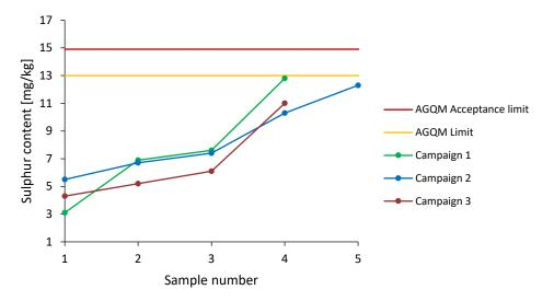
Figure 4: Sulphur content of blend components for biodiesel acc. to DIN EN ISO 20846.
