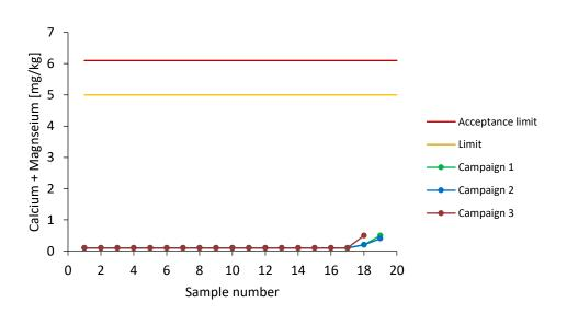
Figure 16: Sum of alkaline earth metals Calcium and Magnesium acc. to DIN EN 14538.
