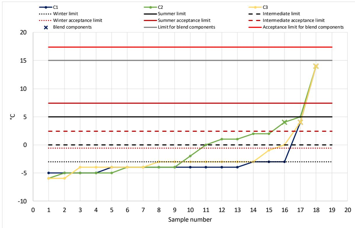
**Diagram 18: Cloud point acc. to DIN EN 23015.**
