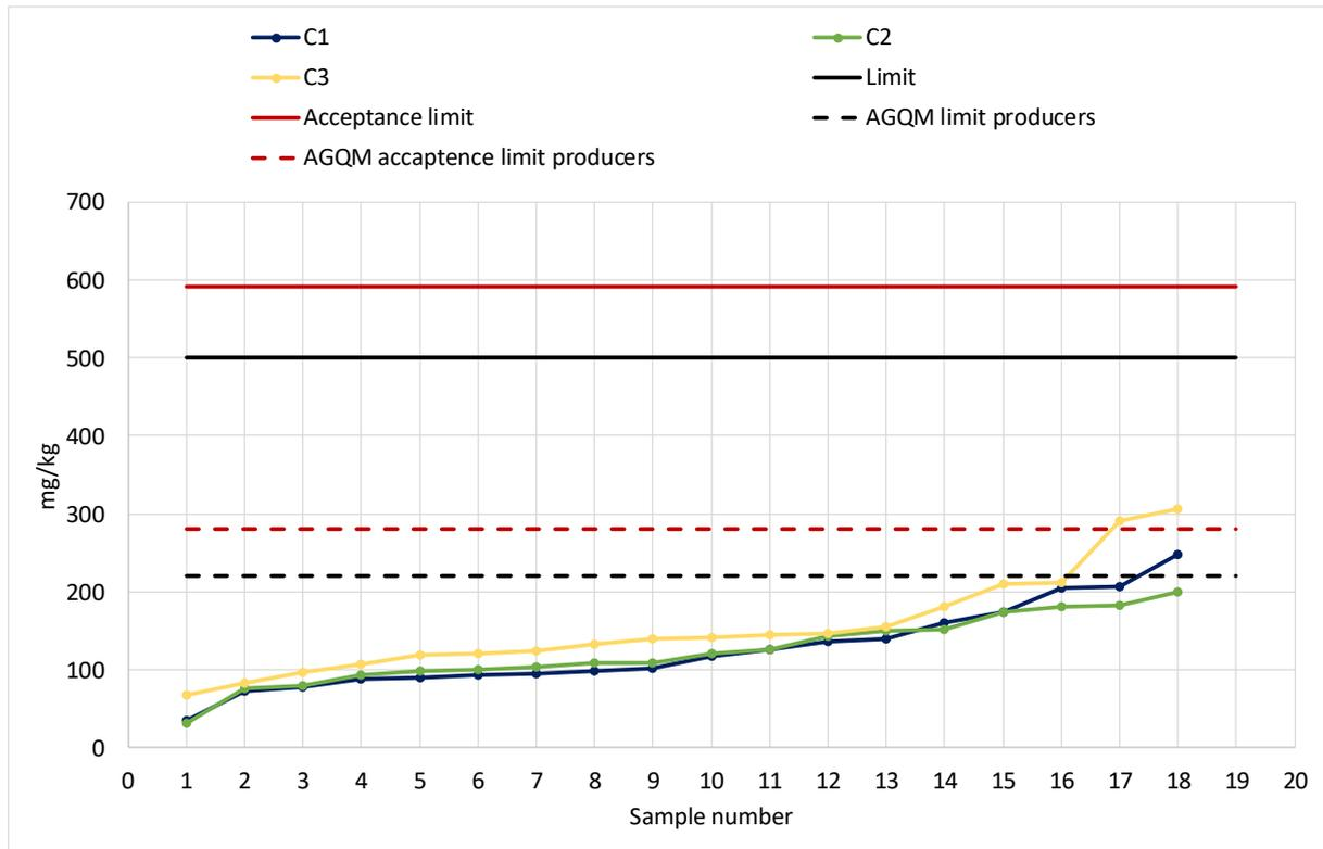
Diagram 4: Water Content acc. to DIN EN ISO 12937.
