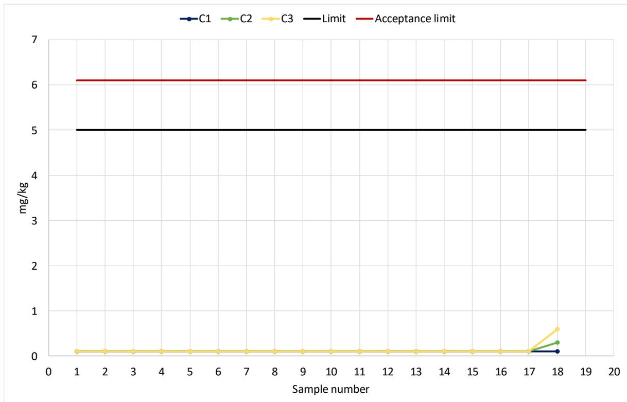
Diagram 14: Sum of Alkaline Earth Metals Calcium and Magnesium acc. to DIN EN 14538.
