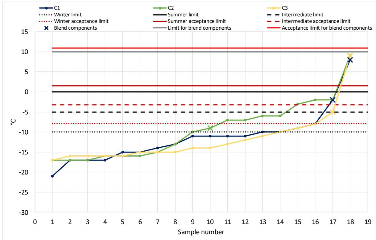
Diagram 17: CFPP acc. to DIN EN 116.
