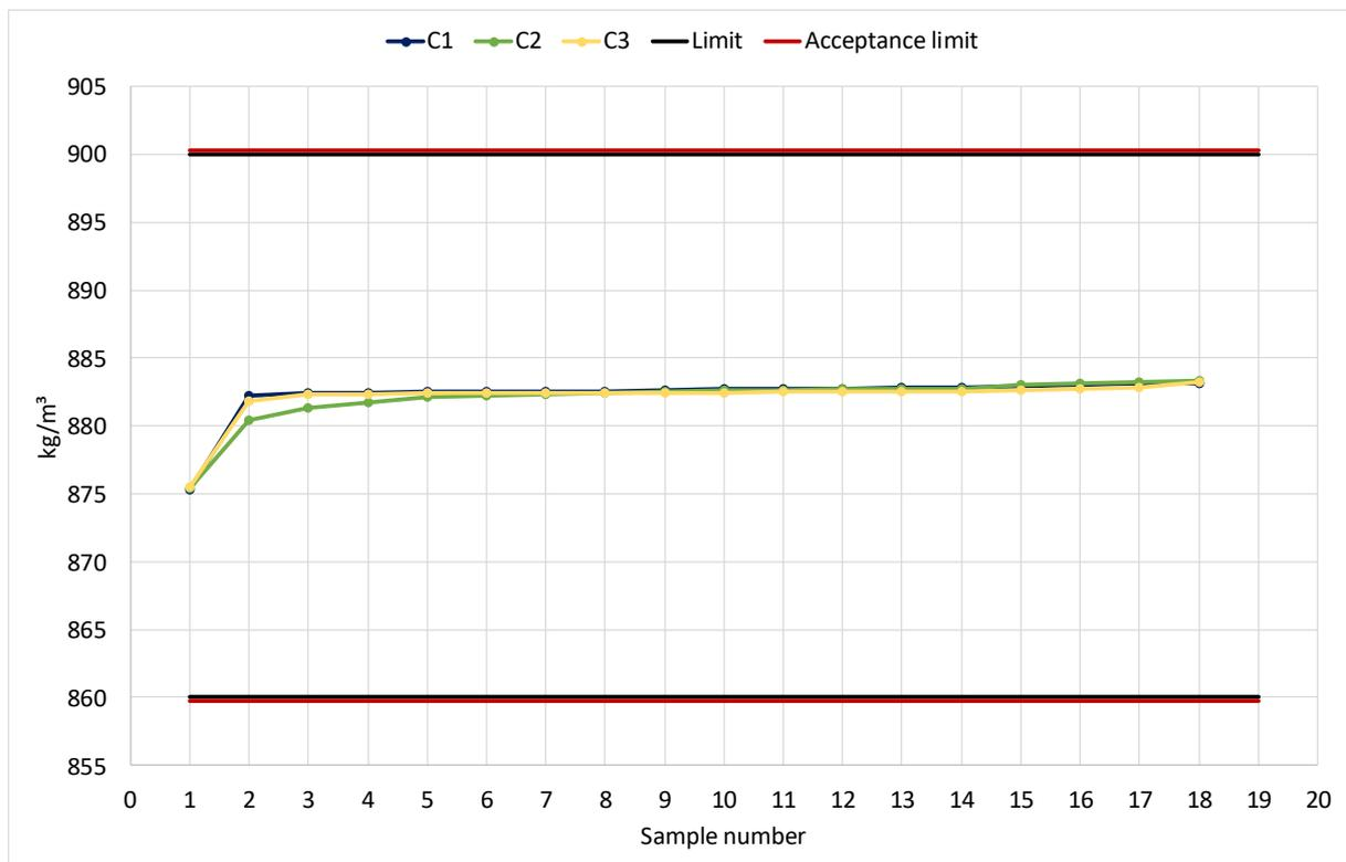
Diagram 2: Density at 15 °C acc. to DIN EN ISO 12185.
