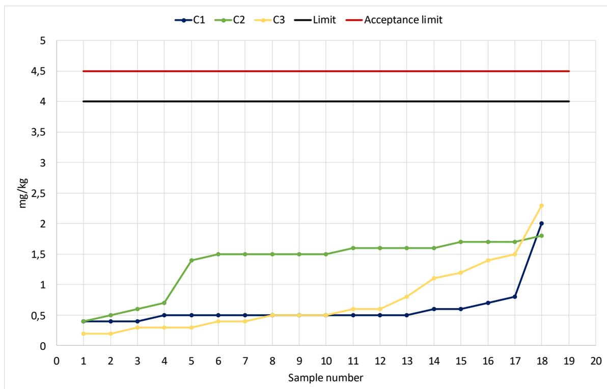
Diagram 15: Phosphorous Content acc. to DIN EN 14107.
