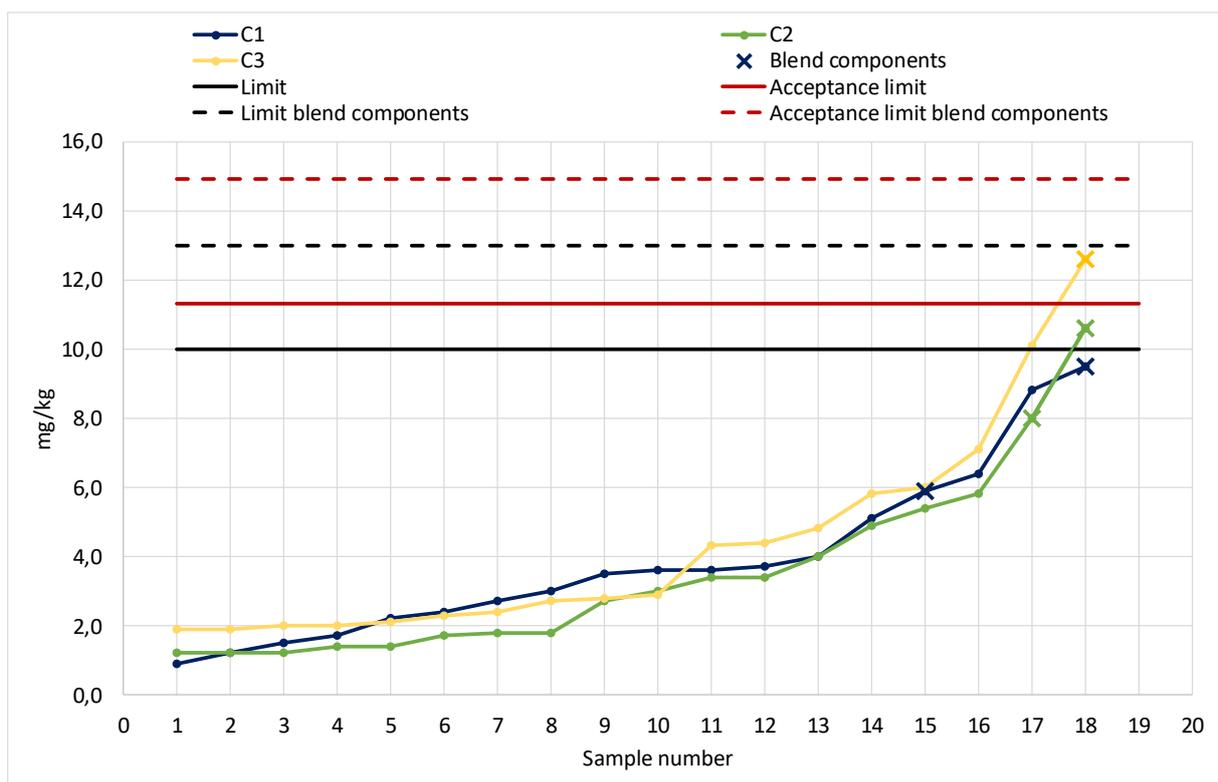
Diagram 3: Sulphur Content acc. to DIN EN ISO 20846.
