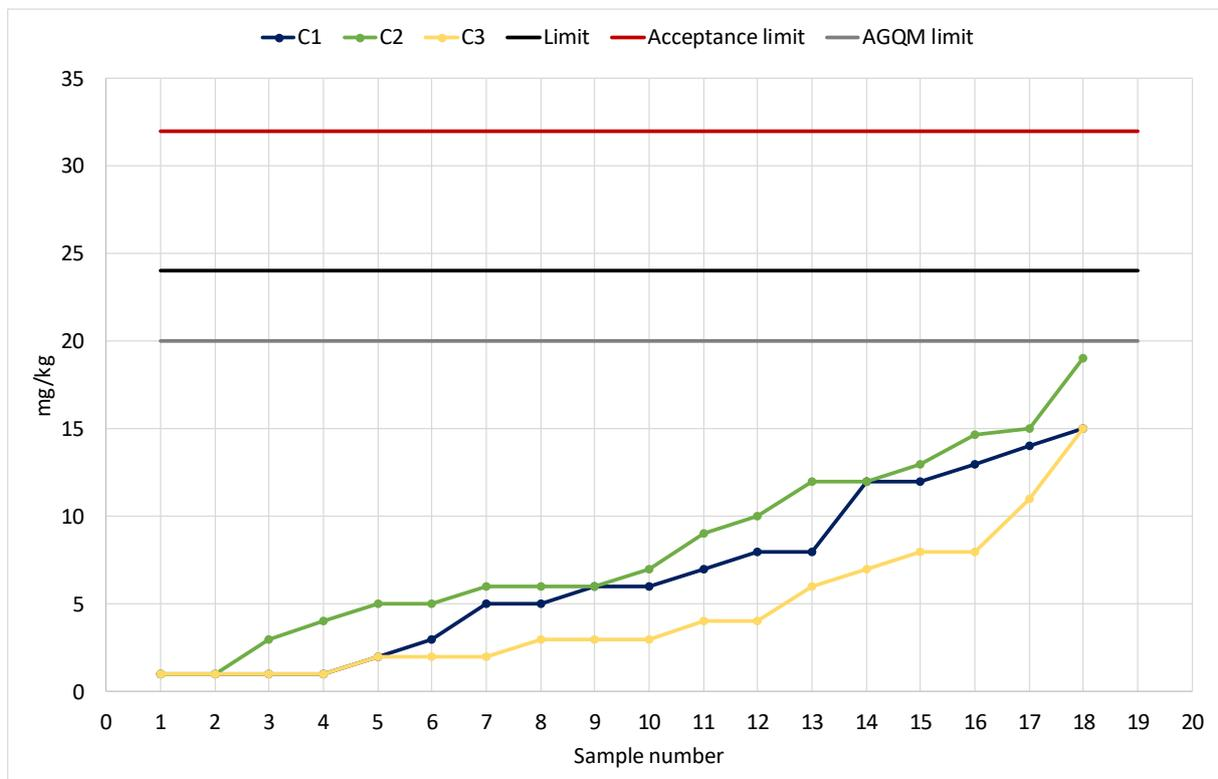
Diagram 5: Total Contamination acc. to DIN EN 12662.
