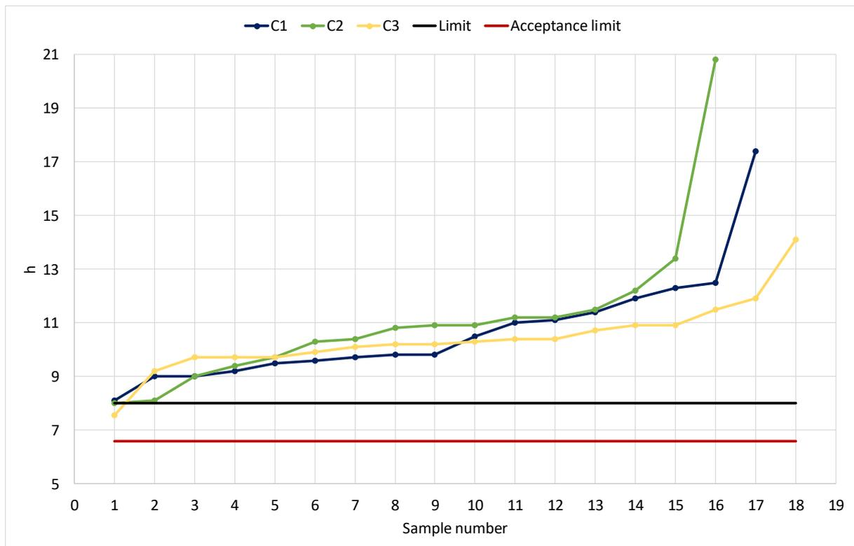
Diagram 6: Oxidation Stability acc. to DIN EN 14112.
