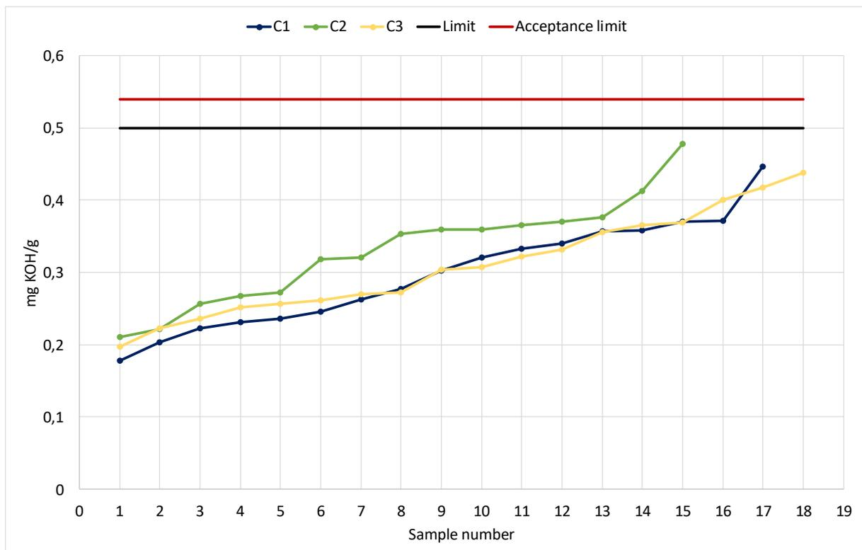
Diagram 7: Acid Number acc. to DIN EN 14104.
