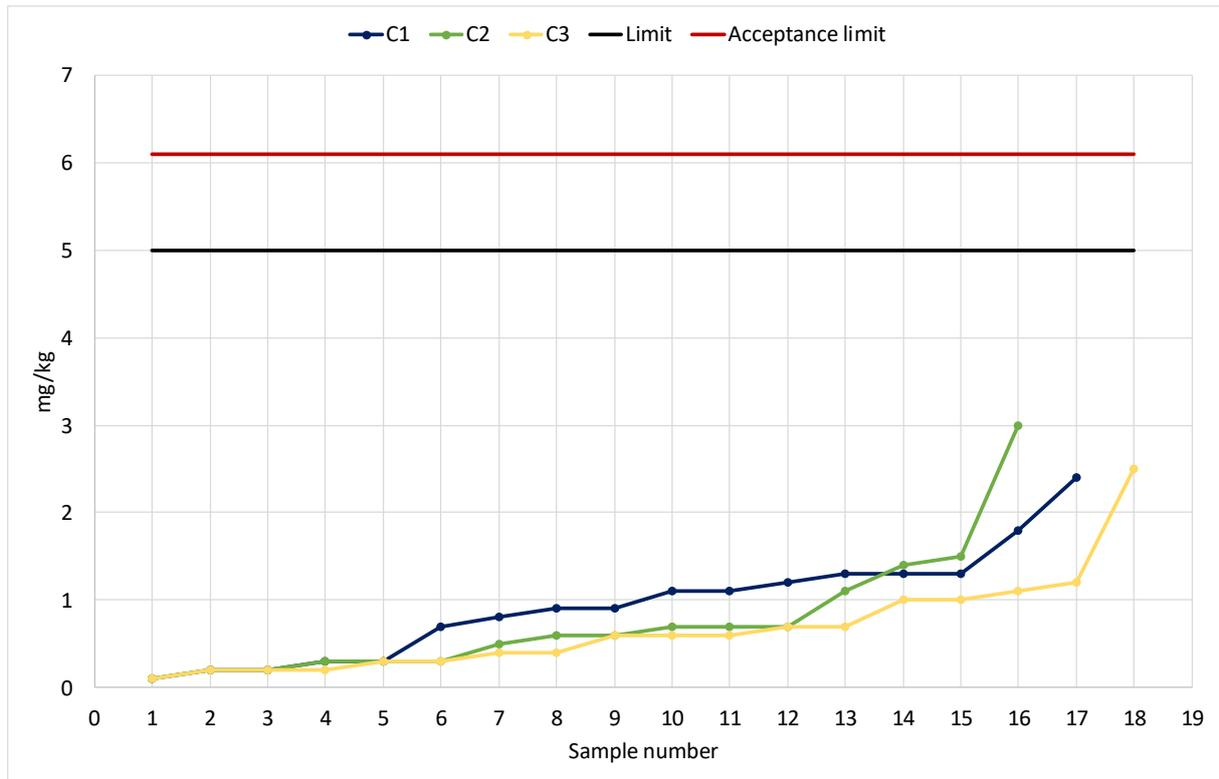
Diagram 13: Sum of Alkali Metals Sodium and Potassium acc. to DIN EN 14538.
