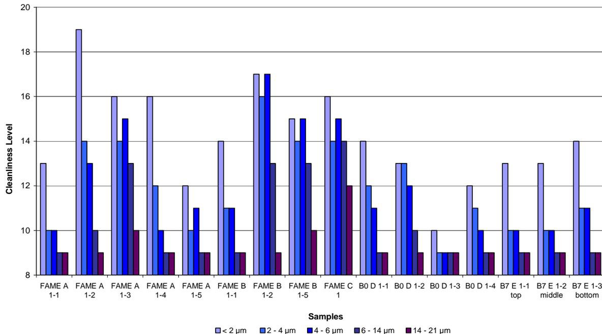
Fig. 3: Classification into Cleanliness Levels of FAME, Fossil Diesel and B7 Fuel Samples
