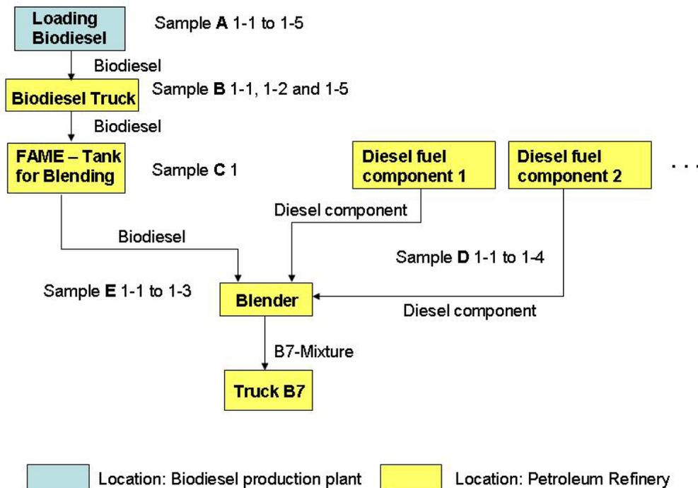
Fig. 1: Diagram of sampling points at Total Deutschland GmbH (supply chain 1)
