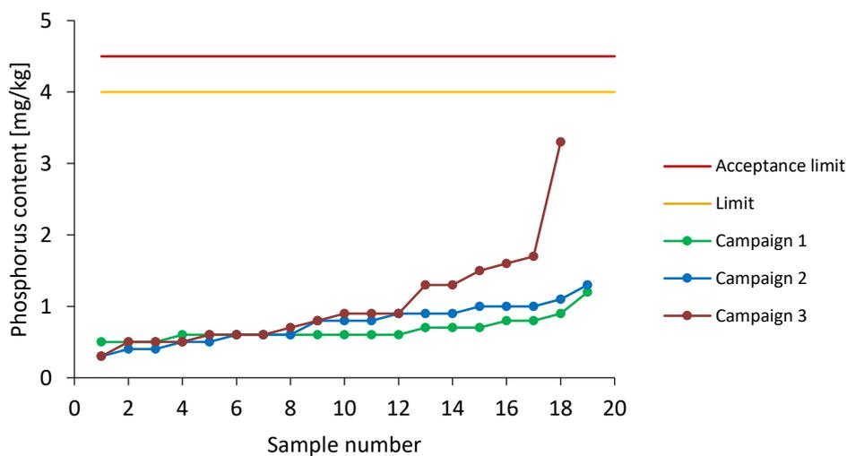
Figure 17: Phosphorus content acc. to DIN EN 14107.
