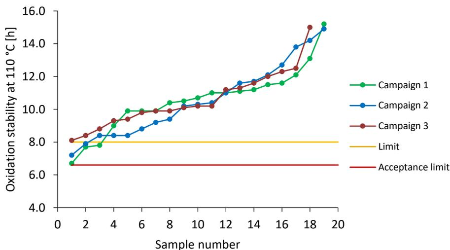
Figure 7: Oxidation Stability acc. to DIN EN 14112.
