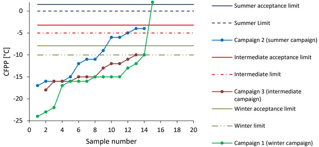
Figure 19: CFPP acc. to DIN EN 116.
